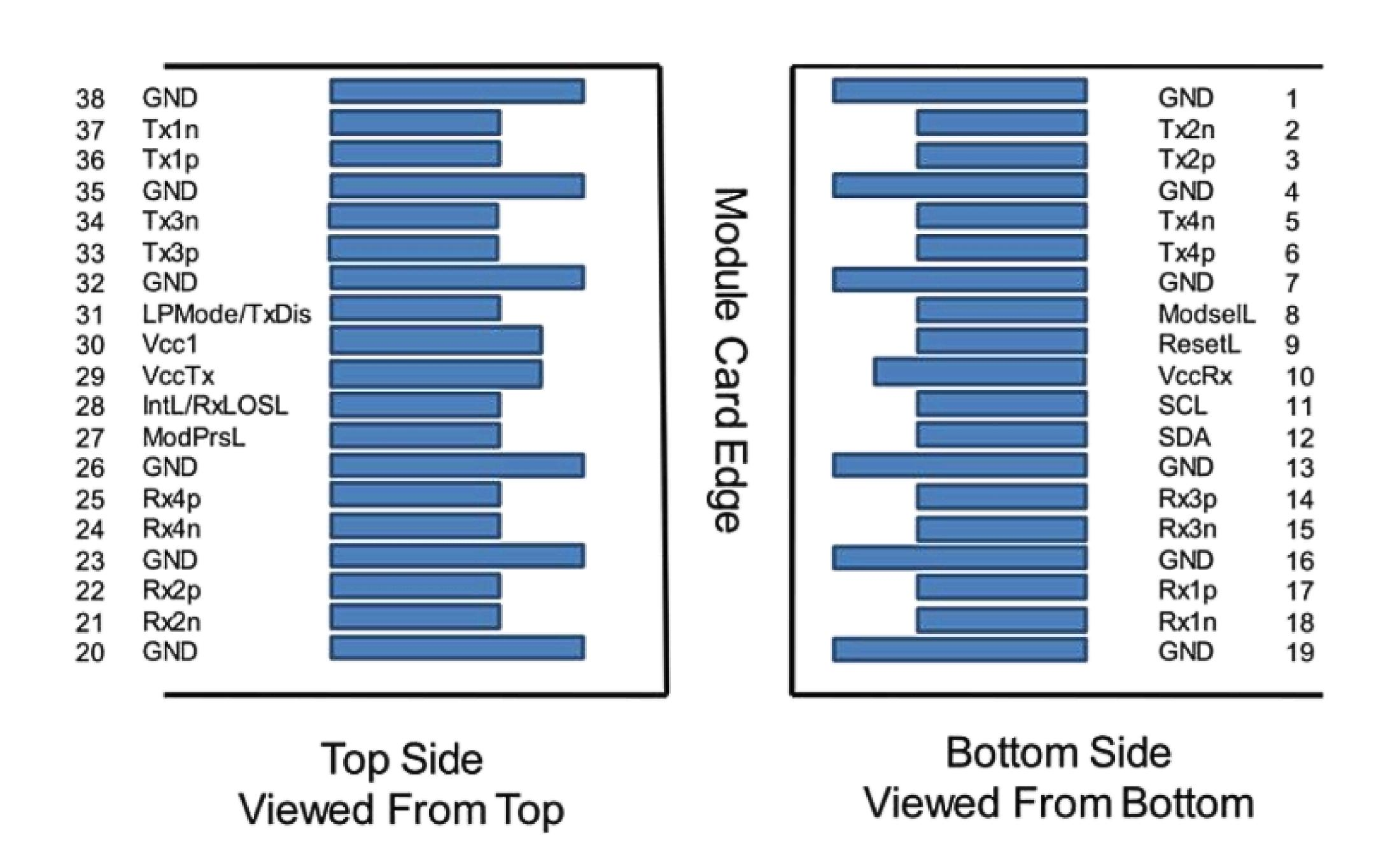
Note 1: GND is the symbol for signal and supply (power) common for the QSFP28 module. All are common within the QSFP28 module and all module voltages are referenced to this potential unless otherwise noted. Connect these directly to the host board signal-common ground plane.
